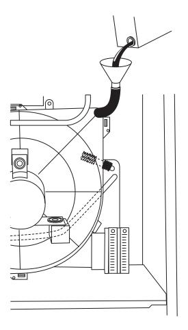
Fig. 55—Filling Condensate Trap
